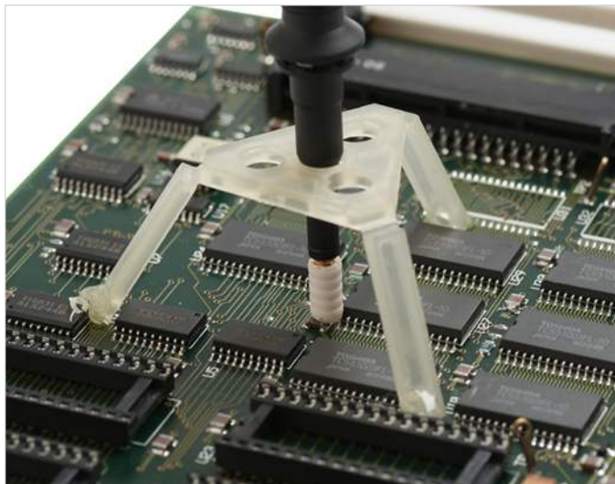
Figure 2.1. Most probes consist of a probe head, a probe cable, and a compensation box or other signal conditioning network.
