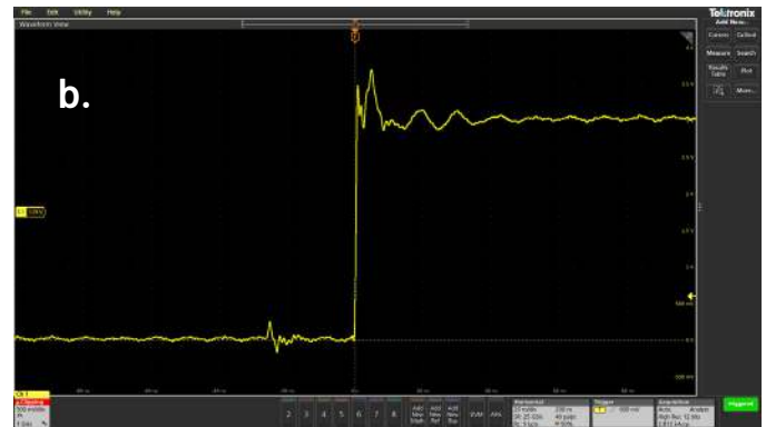
Figure 6.3. A fast step (1.5 ns Tr) has aberrations impressed on it due to use of a 12.5 inch probe ground lead (a). These aberrations can be changed by moving the probe cable or placing a hand over the cable (b).
