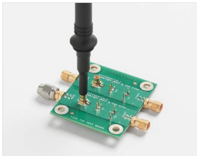
Figure 4.3. A TPP1000 1GHz 10X probe with an MMCX cartridge installed, connected directly to an MMCX connector on a circuit board.
