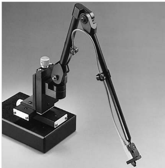
Figure 3.14. Example of a probing station designed for probing small geometry devices such as hybrid circuits and ICs.
