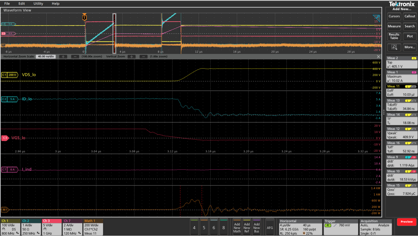
Figure 28: Turn-off parameters and waveforms.
