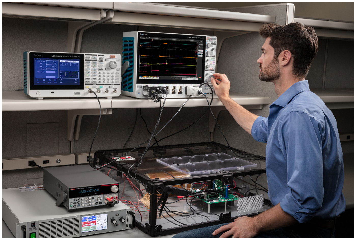
Figure 13: Double pulse test setup for testing a SiC low-side FET, including an MS058B oscilloscope with Double Pulse Testing Application Software, AFG31252 arbitrary/function generator, PSB 11500-06 1.5 kW DC power supply for V_{DD} , and Keithley 2231A-30-3 triple channel power supply to power gate drivers. A T1CP0100 isolated current probe is connected across a shunt resistance to measure drain current. A TCP0030A clamp-on current probe is used to measure the inductor current. In this setup the source of the low-side FET is grounded allowing the use of earth-referenced probes. A TPP0850 high-voltage passive probe is connected to V_{DS} and a TPP1000 passive probe with MMCX cartridge is connected to V_{GS} .
